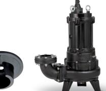
The C-series is a submersible cutter pump for sewage and wastewater, which is made of casting and equipped with cutting mechanism. Featuring a combination of impeller vane with brazed sintered tungsten carbide alloy edge and a suction cover of serrated shape, the C-series pumps enable smooth pumping, while cutting fibrous foreign objects during suction.
