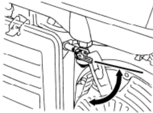
Figure 4-3: Fuel Shutoff Valve
